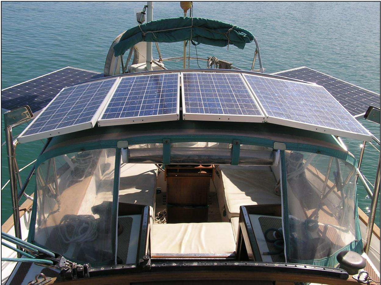
With 453 watts of solar power in 6 panels on *¿Qué Tal?*, we almost never run the diesel just to charge the batteries. Even though one or two panels are frequently shadowed, having so many panels means that the majority of panels are usually putting out power. Our only maintenance is to wipe them off with a damp rag every few days.
